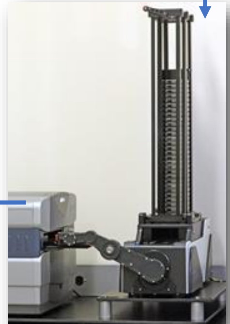
Celigo (Nexcelom) image cytometer with stacker
